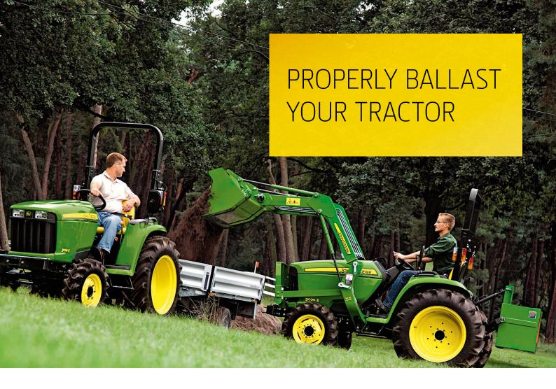
Correct ballasting delivers maximum tractor performance as it helps to put more power to the ground, improving fuel consumption, traction and ride comfort. How much ballast you should use depends on the tractor's horsepower, the speed it needs to move at and the type of implement being used.
