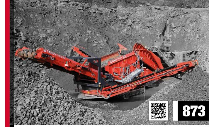
The NEW Terex Finlay 873 is ideally suited to working in aggregates, sand and gravel, top soil, construction demolition and recycling applications. This highly versatile machine can be fed either by a tracked mobile crusher, shovel or an excavator and has the capacity to process at a rate of up to 450 Tonnes per hour.
