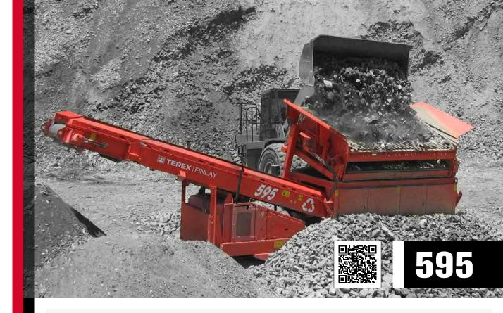
The Terex Finlay 595 Hydratrak is a self contained high capacity mobile scalping unit. Designed and constructed to the highest specification, the 595 can withstand the toughest of applications from waste reclamation projects to quarry face and demolition environments, special features include a heavy duty twin deck vibrating grid, remote control movement and a tracked undercarriage.
